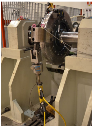
Figure 7 Lucchini RS test facilities (above and below), showing the TX4 wheel resilient wheel assembly during type testing to verify the wheel stiffness in radial, lateral and torsional direction in new and artificially aged condition.
