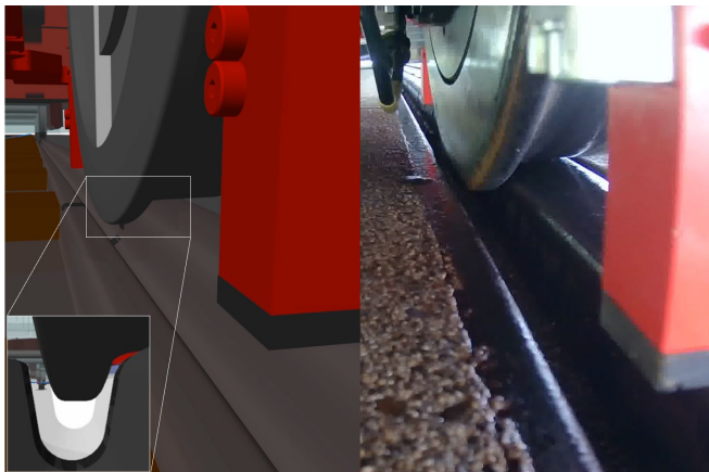
Figure 10 The TX4 on the tracks in Zürich, showing the Lucchini RS wheel in the center of the tram track groove (1m gauge) in addition to the Traila
