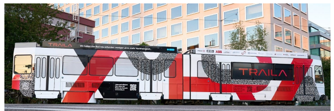
Figure 1 TX4 (Traila T2000 Test Tram) currently being tested on the tracks (1m gauge) at VBZ Zentrum, Zürich
